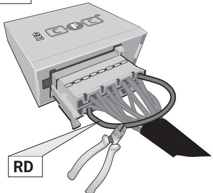
Pin 11 and Pin 2 disconnected
