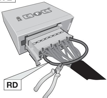
**Pin 11 and Pin 2 disconnected
